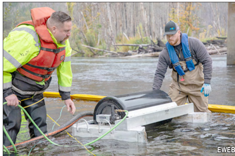
Steve Brown (City of Springfield) left, and Brady Shaw on the right (SUB) are operating the floating drum oil skimmer.
