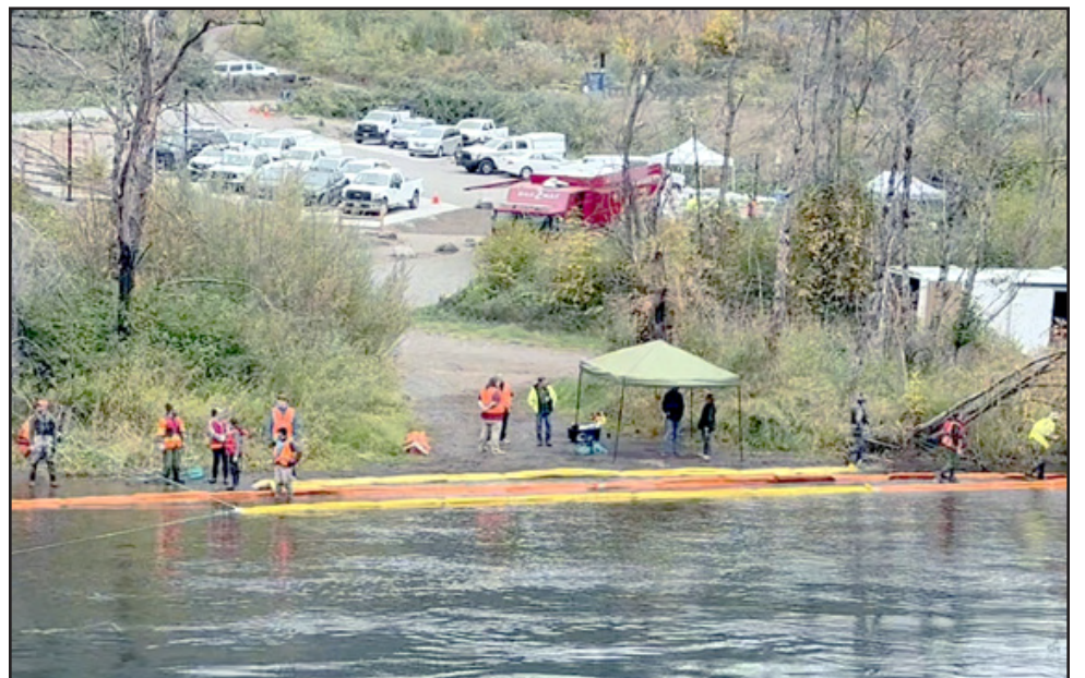
During simulations at the Finn Rock Landing, crews used floating booms that direct surface contaminants like oil into a skimmer to remove pollutants from the water.
