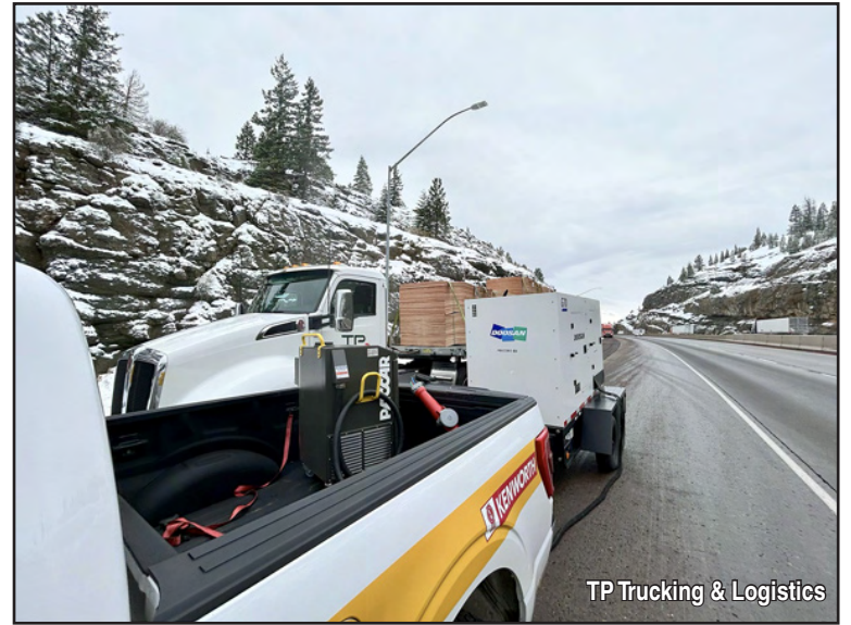
Out of Juice: A mobile diesel generator recharges an electric truck that stalled atop the Siskiyou Summit.
